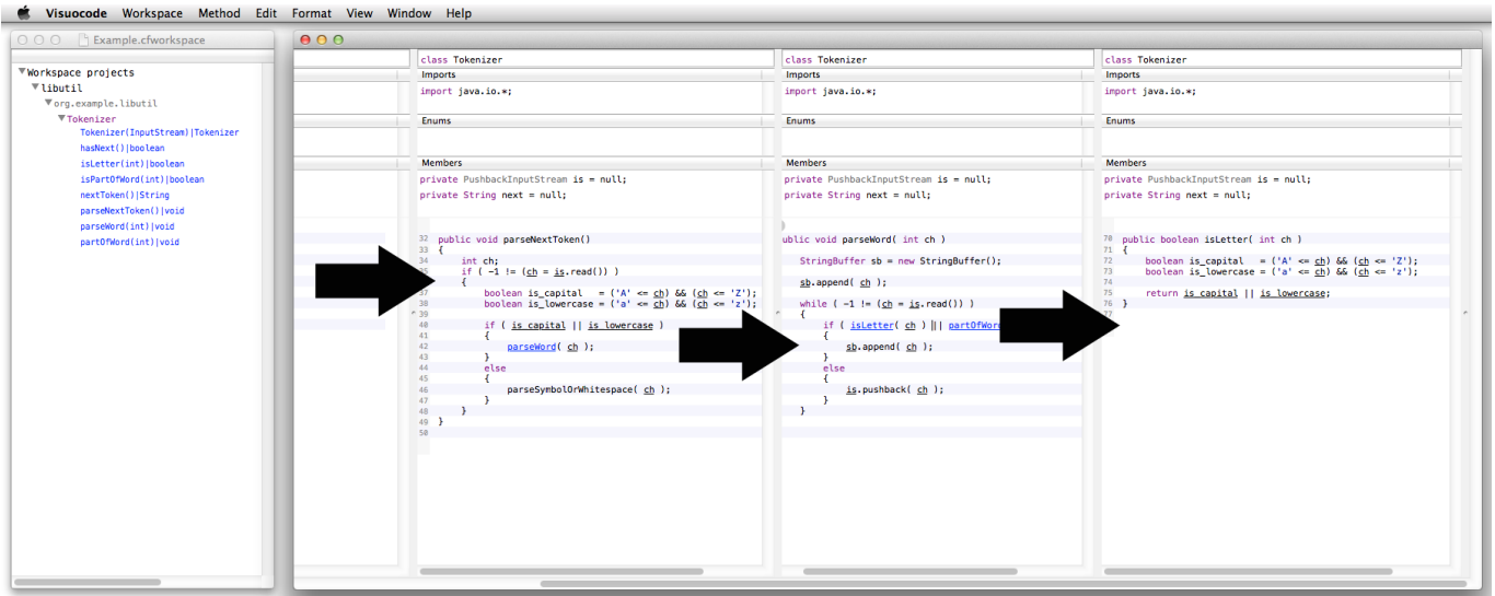
Fig. 2. Visuocode consists of two types of window: the workspace manager (left), and the flow window (right). The workspace manager is used to manage projects and set the left-most editor column of the flow window. The flow window implements method-flow by allowing an arbitrary number of editor columns to be contained within a scrollable flow view . In the image above, the programmer selected the nextToken method, then navigated to the parseNextToken method, the parseWord method, then finally the isLetter method (see Fig. 3 for a closer look).
